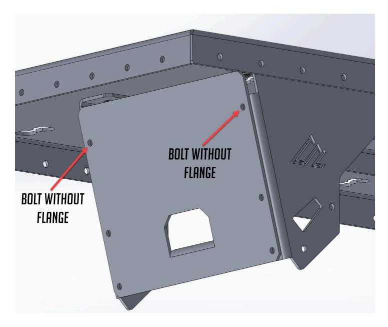
Then, using (4) 6mm x 20mm flange head bolts, secure the alignment tabs to the end caps as shown below. Be careful to position the flanges on the alignment tabs as they are shown in the diagram below.
