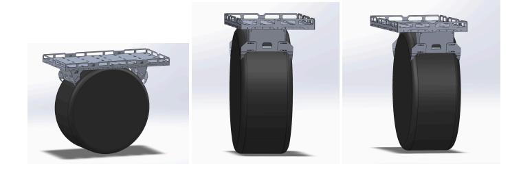
Center the vertical brackets on the tire (front to rear) and ensure that the main platform is level.
