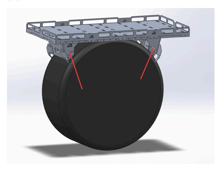
Ensure that the straps go all the way through the platform and then through the wheel. The red line below illustrates the path for the straps.
