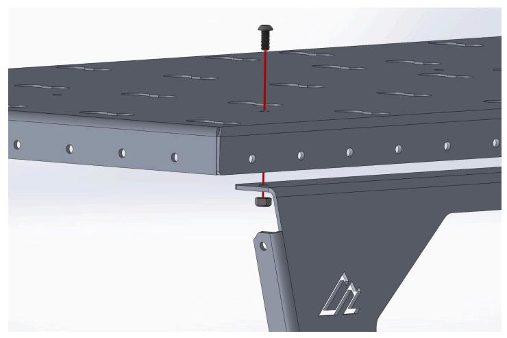
After both vertical brackets are loosely installed, here's what it should look like.
